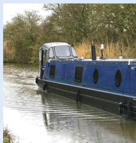
A combination of steel dodger and well-fitted canopy extends the living space and is practical when cruising on many navigations.
